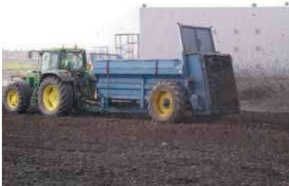
Spreading organic matter onto subsoil
