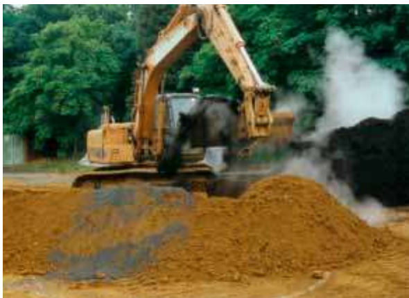
Blending organic matter with mineral material
