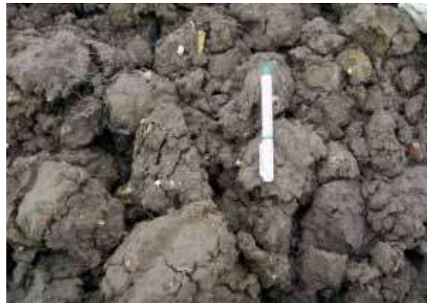
Damaged, heavy clay natural topsoil
